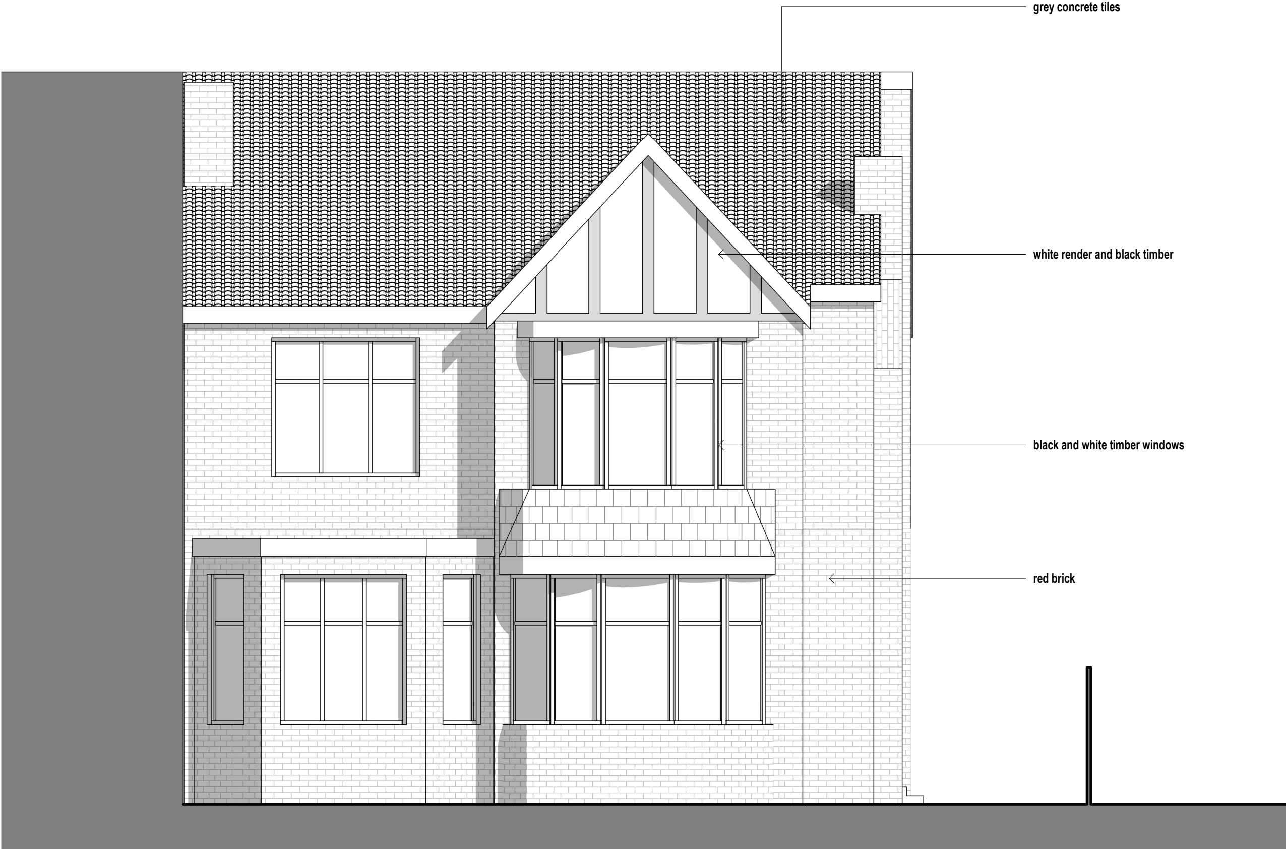
EXISTING ELEVATIONS - FRONT 1 : 50
