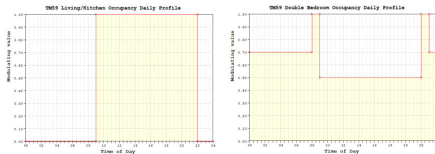
Figure 8. Kitchen/Living/Dining and Double Bedroom Modulating Profile for Occupant Gains
