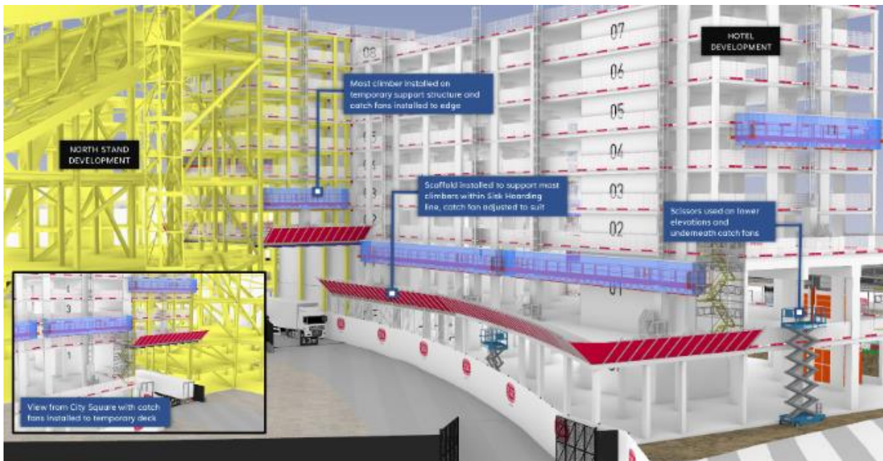
Diagram 8E – Fall Protection Proposal
