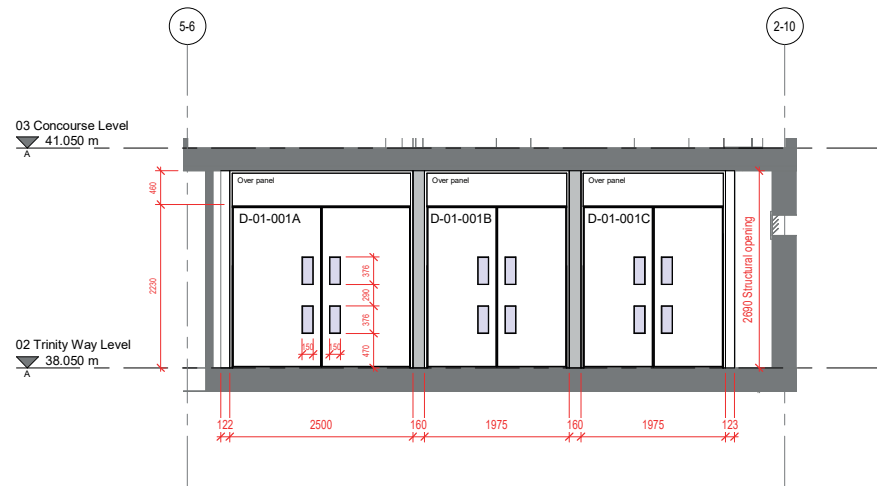
2 Tunnel Entrance Elevation From Trinity Way 1 : 50
