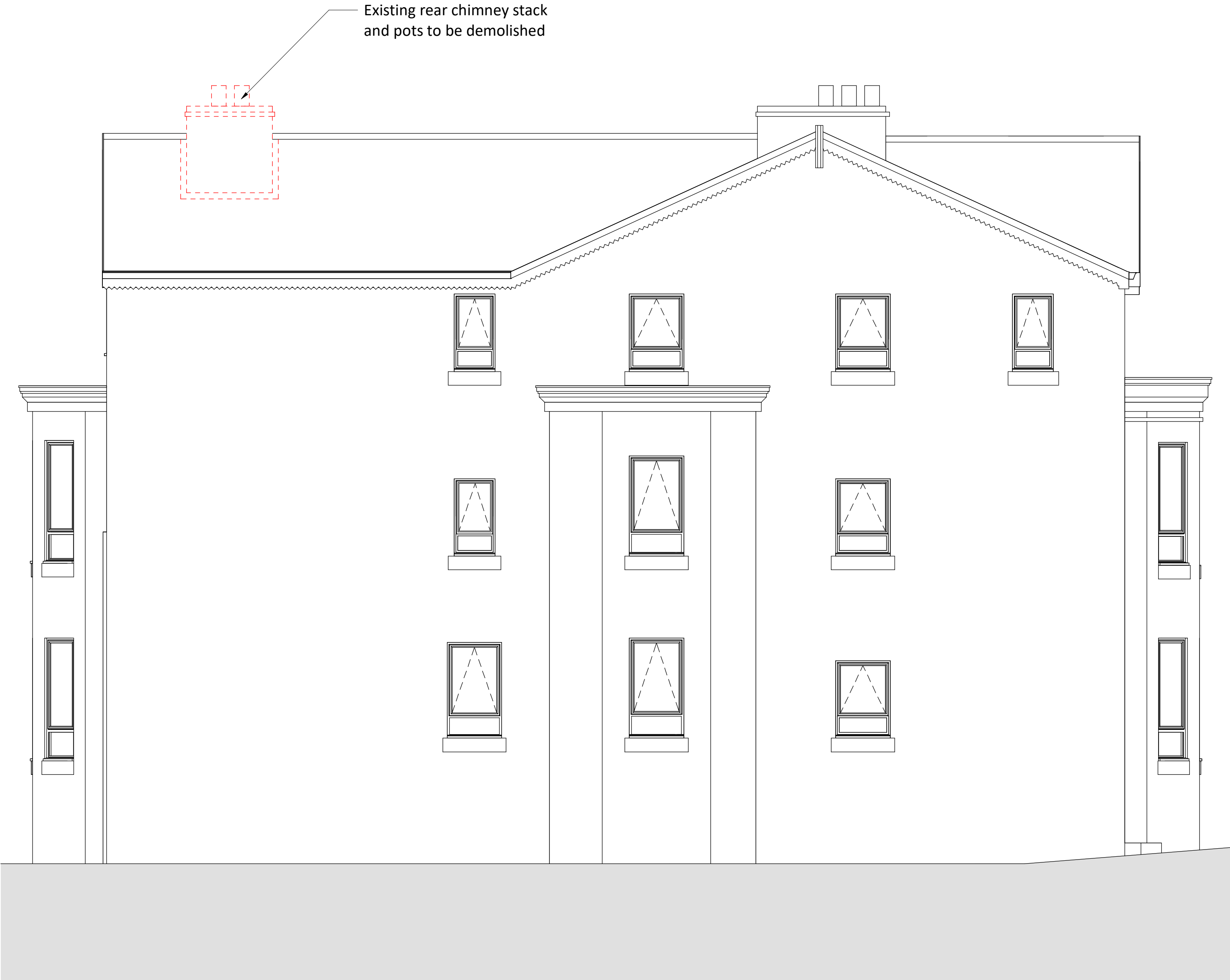
Gable Elevation Demolition 1 : 50
