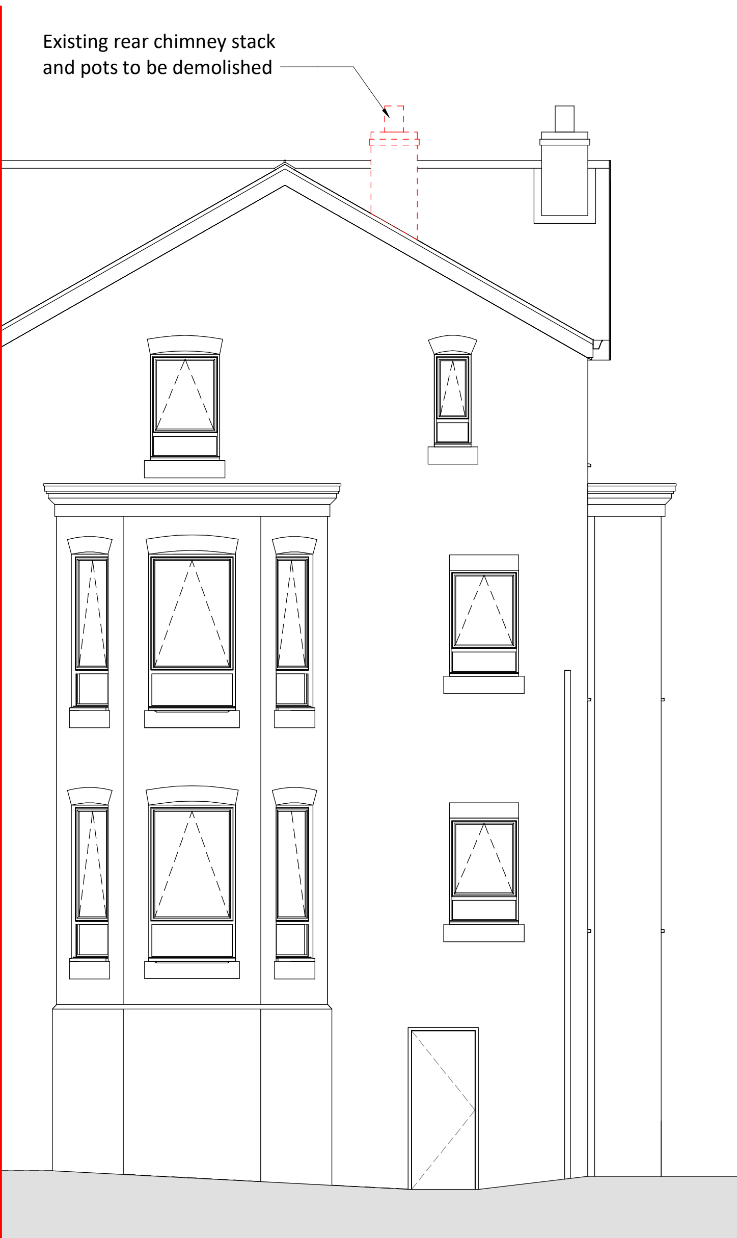
Rear Elevation Demolition 1 : 50
