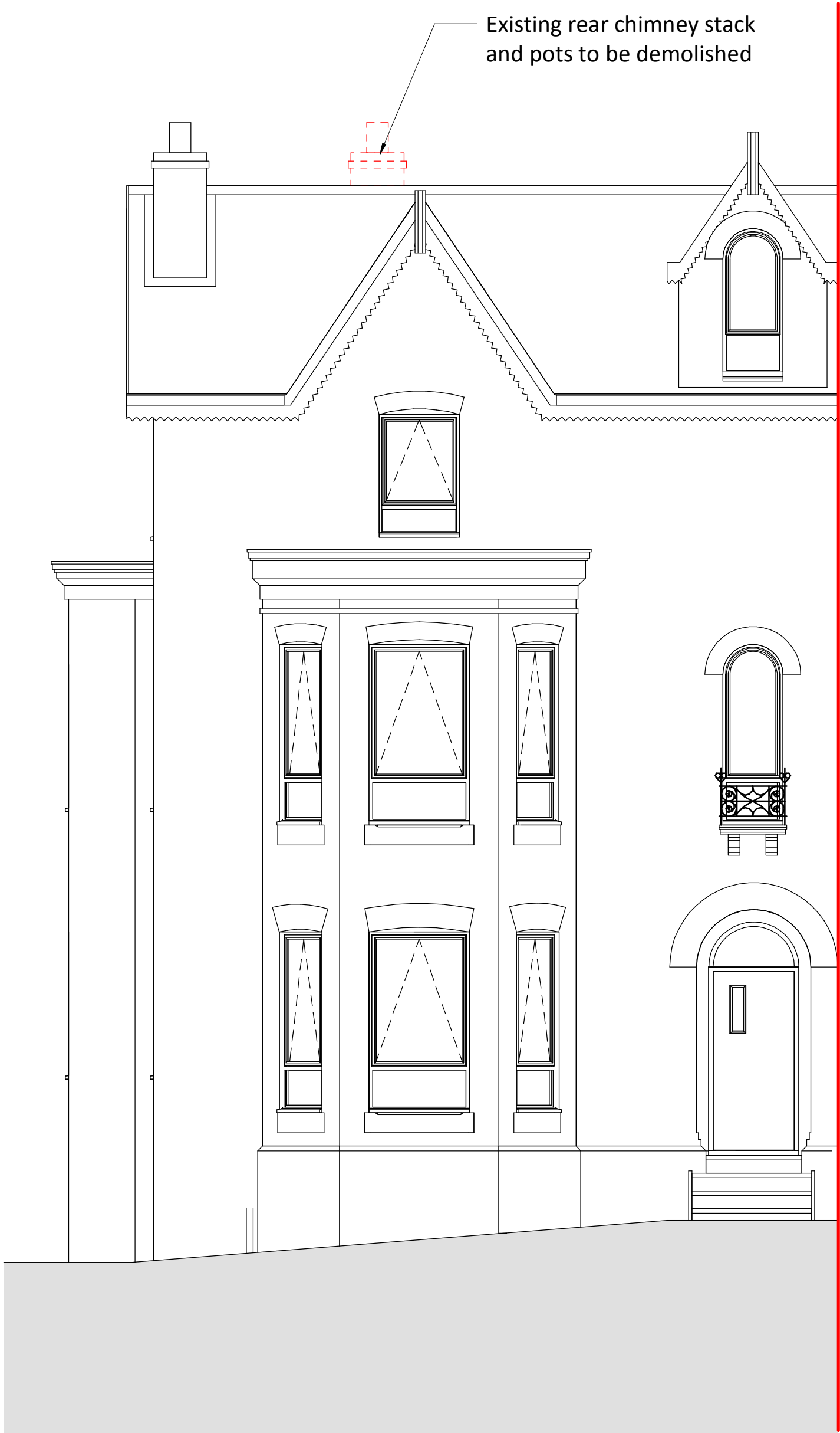
Front Elevation Demolition 1 : 50
