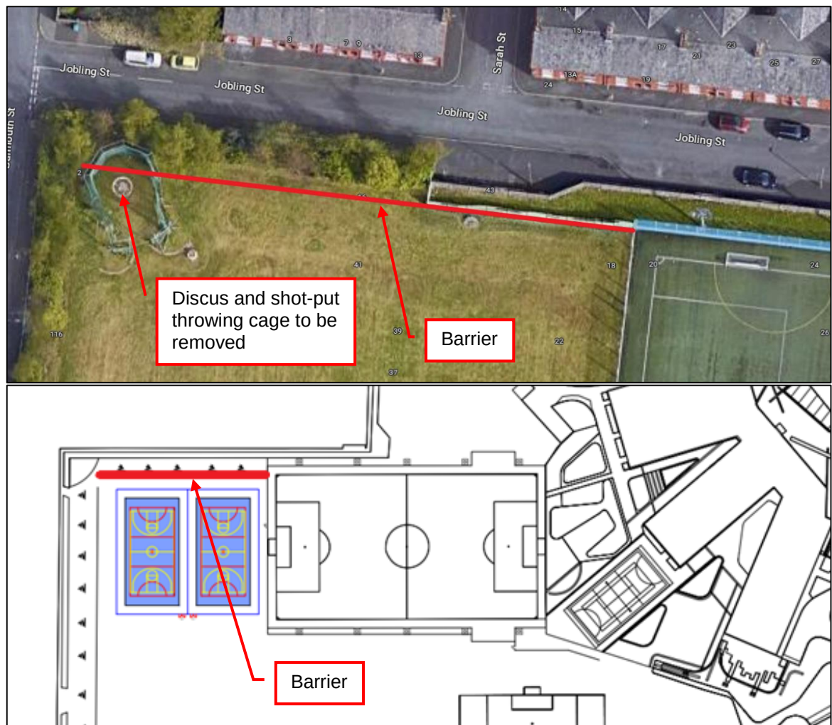
Figure 4.2 - Potential noise barrier location
