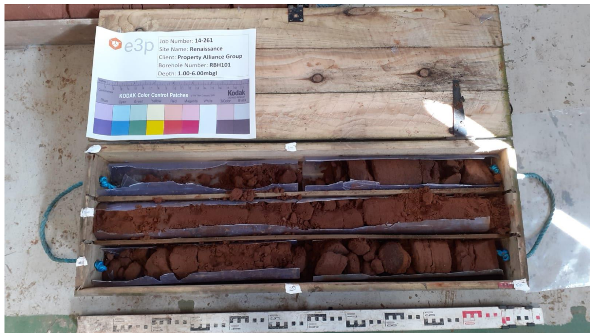
PLATE 3 RBH101 ROCK CORE (1.00 – 6.00 M BGL)
