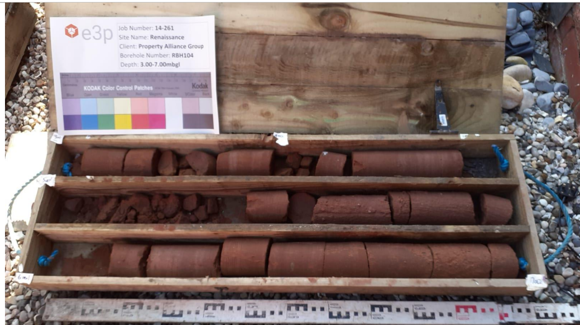
PLATE 5 RBH104 ROCK CORE (3.00 – 7.00 m bgl)
