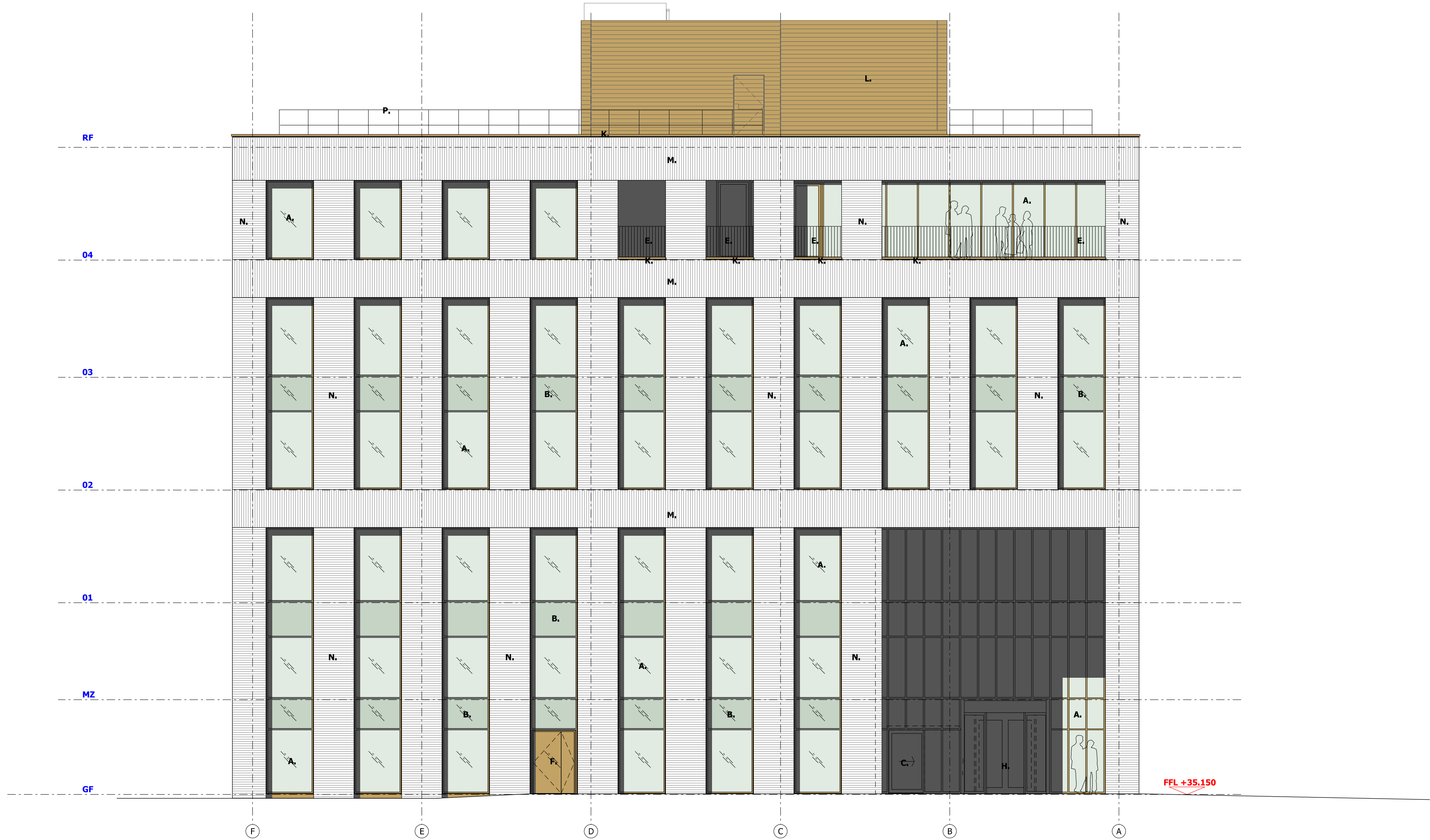
EXISTING EAST ELEVATION (1:100)
