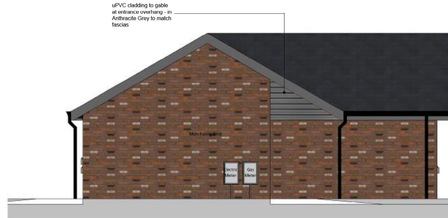
04 Gable Elevation 2 Brick Type B 1 : 50
