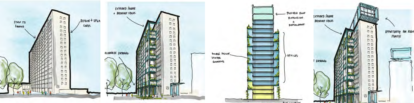
Fig 85 Retaining and extending 18 storey building, scenario 1
