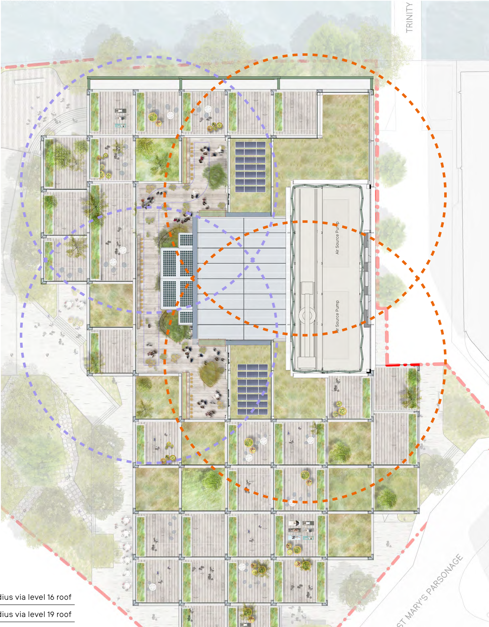
Fig 349 Roof Plan showing BMU tracks on levels 16 and 18
