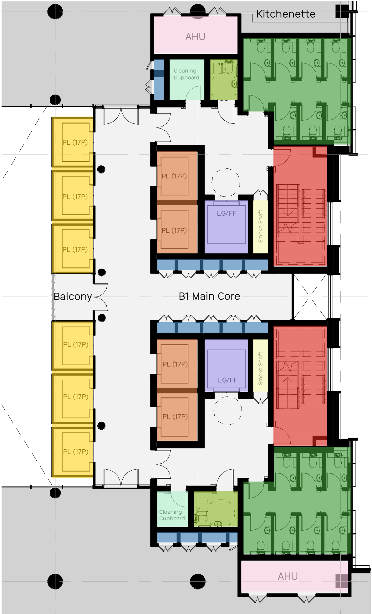
Fig 274 Level 4 - Main Core Diagram
