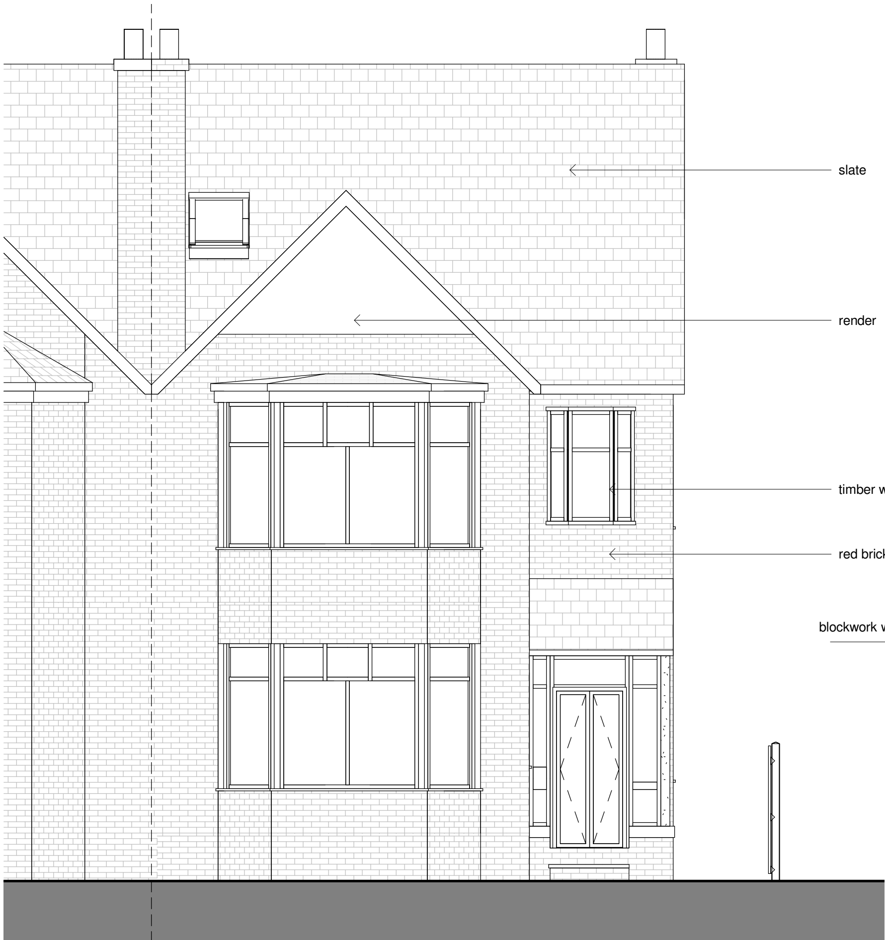
EXISTING ELEVATIONS - SOUTH 1 : 50
