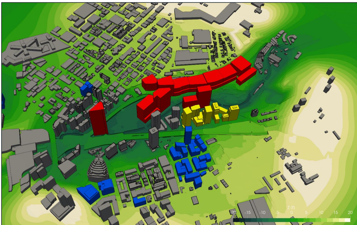
Figure 2-5 - Screenshot of the CAD model for the Outline Masterplan, detailed NT02-04 developments and cumulative schemes, showing the level of detail in the model.
