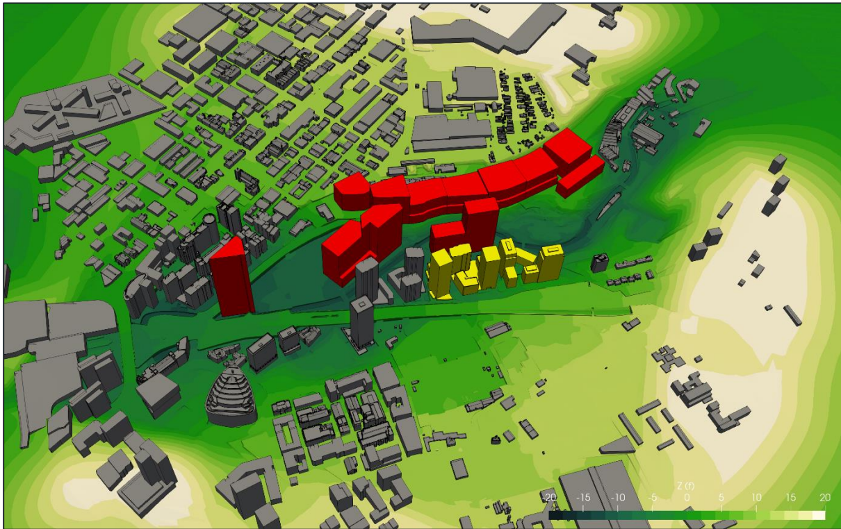
Figure 2-5 - Screenshot of the CAD model for the Outline Masterplan, detailed NT02-04 developments and cumulative schemes, showing the level of detail in the model.
