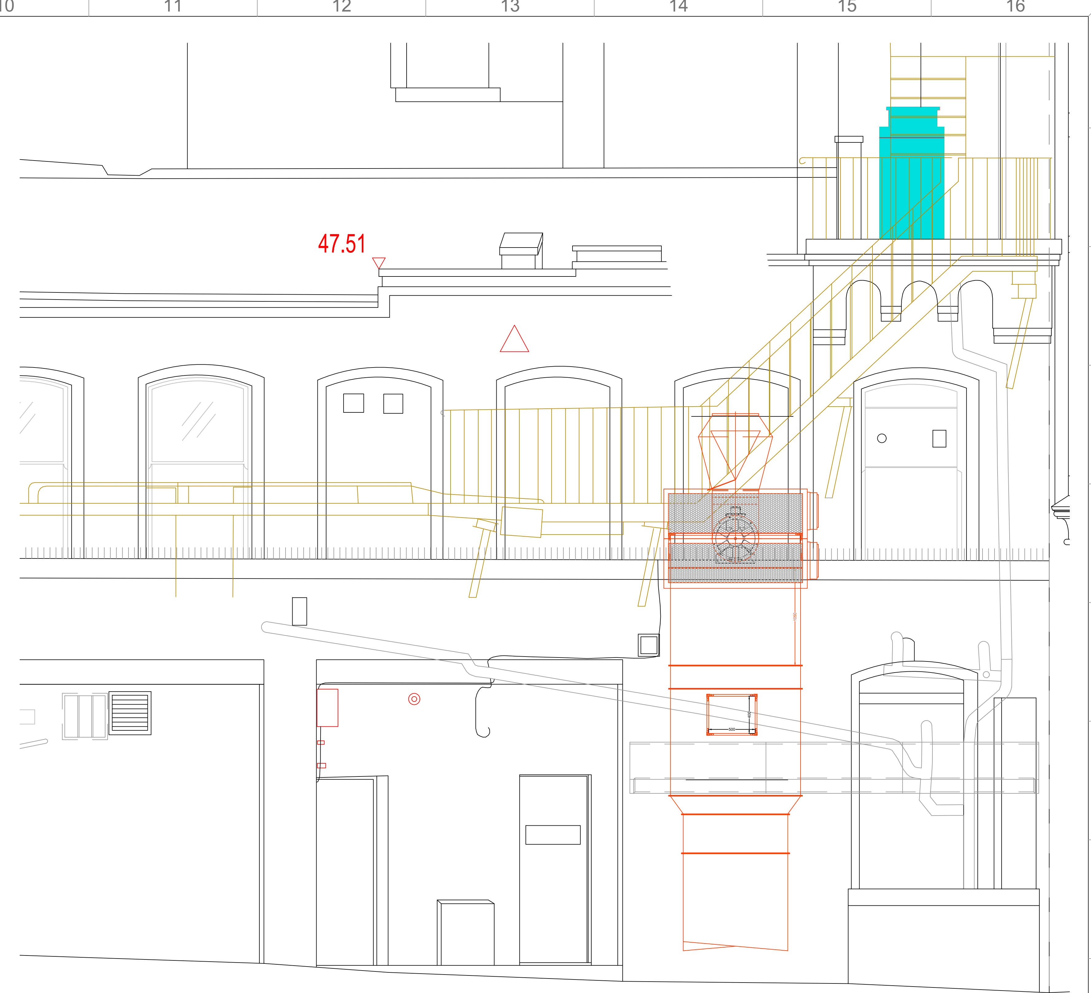
EXTRACT AND AIR SUPPLY DUCT INSTALLATION AS VIEWED ON BOW LANE
