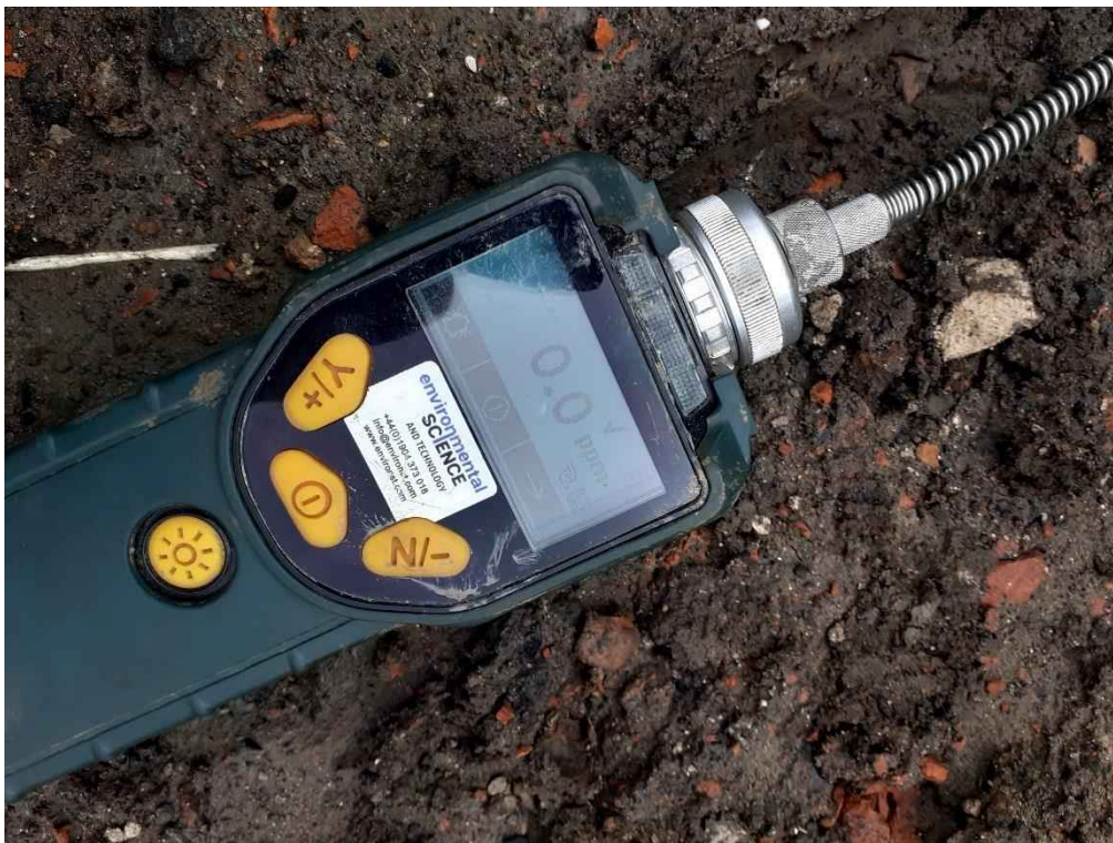
PLATE 8 PID SCREENING OF MADE GROUND DURING TURNOVER
