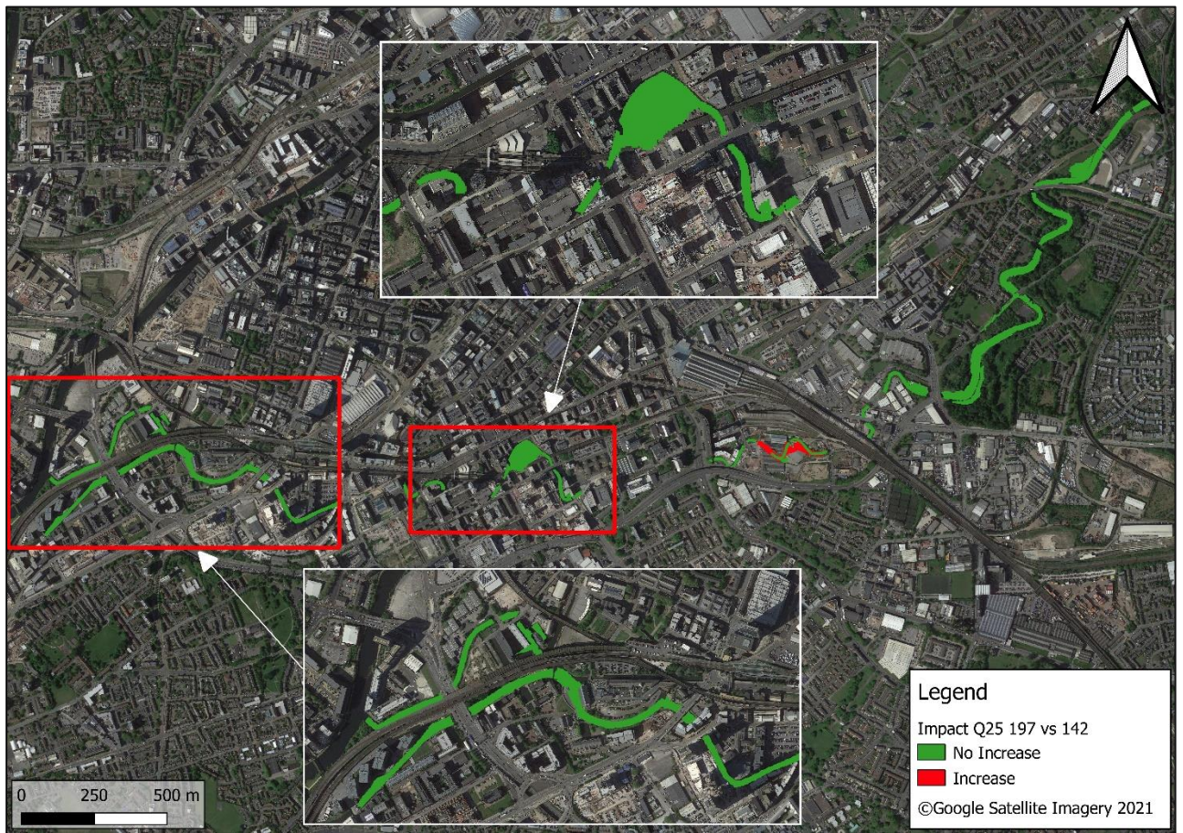
Figure 3-12: Impact on flood extent as a result of the amended Full Build Out Model (197) for the 1 in 25 year return period event
