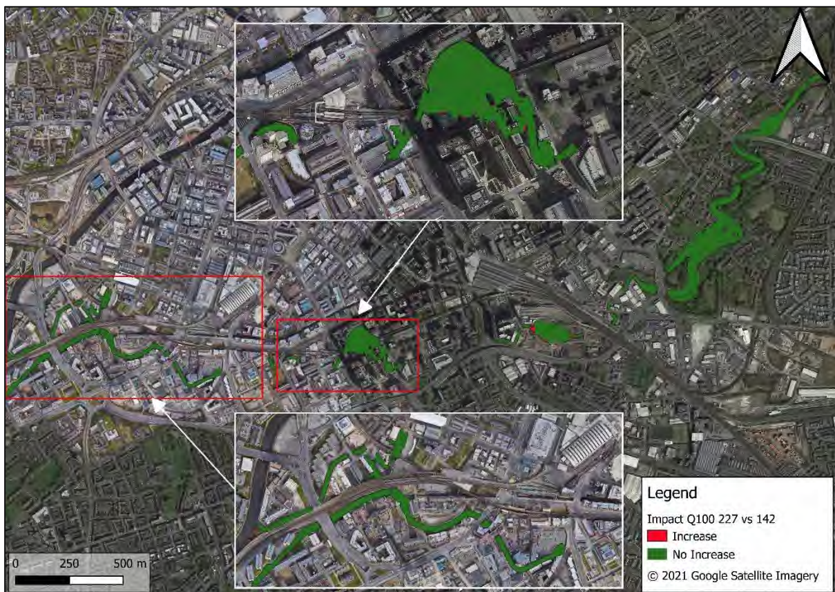
Figure 3-13: Impact on flood extent as a result of the amended Design Changes Model (227) as compared to the BHE Baseline 2020 model (142) for the 1 in 100 year return period event
