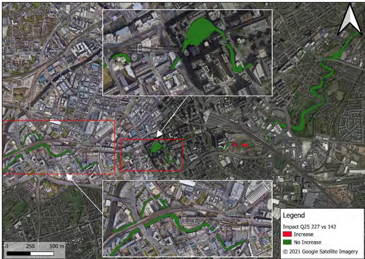
Figure 3-12: Impact on flood extent as a result of the amended Design Changes Model (227) as compared to the BHE Baseline 2020 model (142) for the 1 in 25 year return period event
