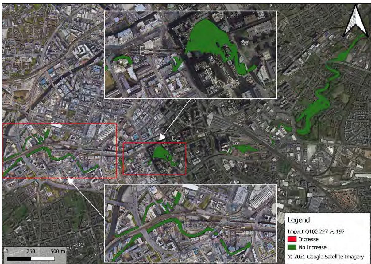
Figure 3-7: Impact on flood extent as a result of the amended Design Changes Model (227) as compared to the Full Build Out Model (197) for the 1 in 100 year return period event
