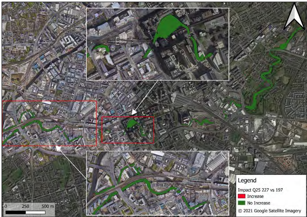
Figure 3-6: Impact on flood extent as a result of the amended Design Changes Model (227) as compared to the Full Build Out Model (197) for the 1 in 25 year return period event
