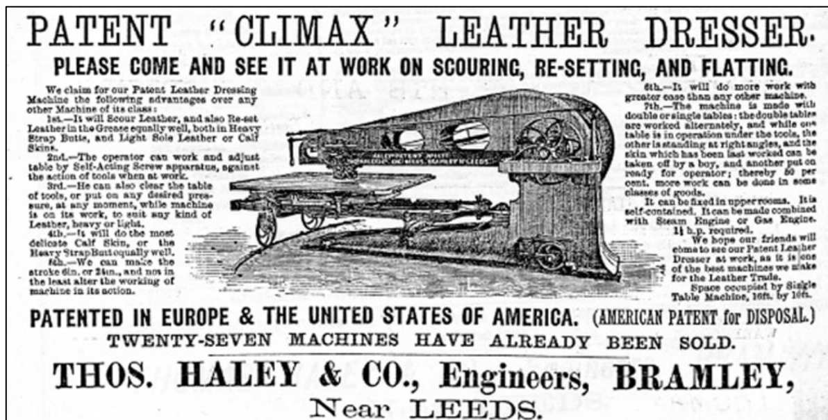
Plate xx: 1890s example of a 'Scouring Machine' by Haley & Co. of Leeds, who held the patent for 'Jacksons Scouring Machine'
