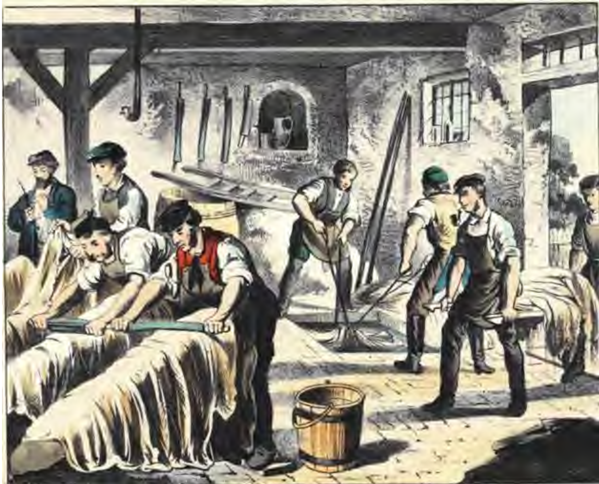
Plate xx: Image illustrating the process of scouring in a late 19 th century tannery (Courtesy of the Hagen History Centre)
