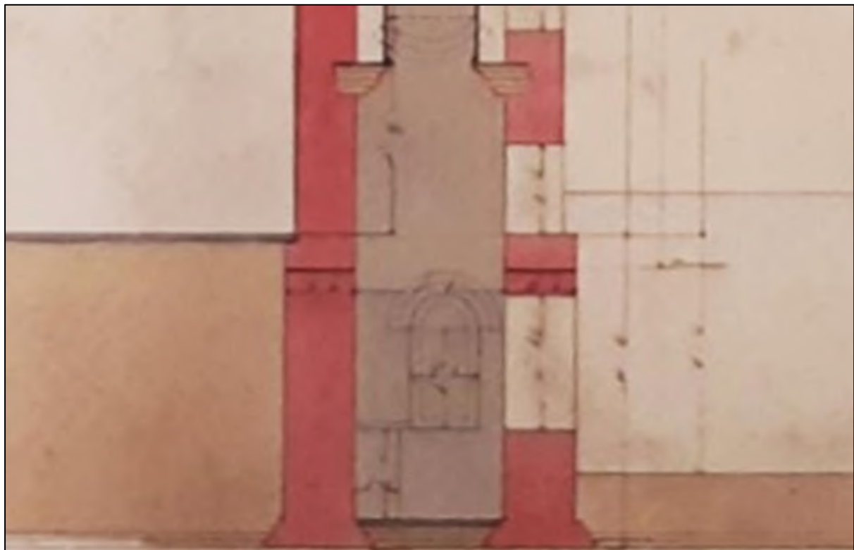
Plate 185: Detail of chimney foundation illustrating the position of the flues
