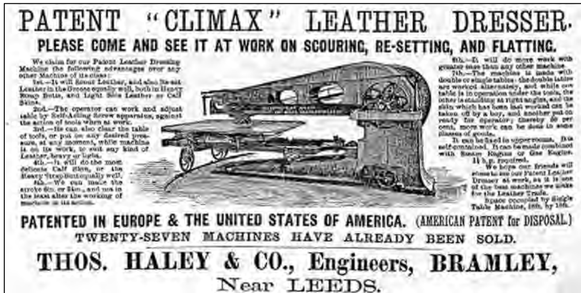
Plate 176: 1890s example of a 'Scouring Machine' by Haley & Co. of Leeds, who held the patent for 'Jacksons Scouring Machine'
