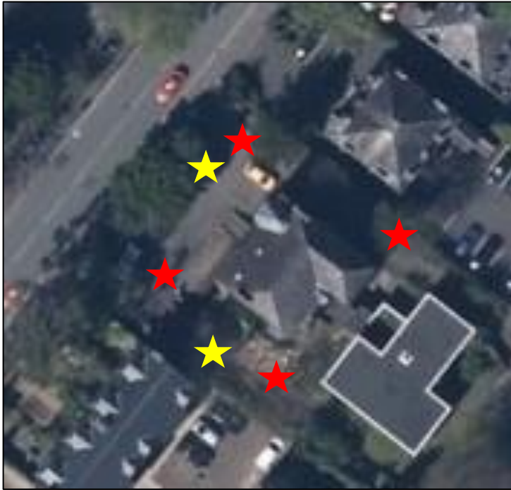
Figure 2 showing the locations of the surveyors (red stars) and the location of the infra-red and thermal cameras (yellow stars)
