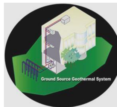
Ground Source Heat Pump Installation
