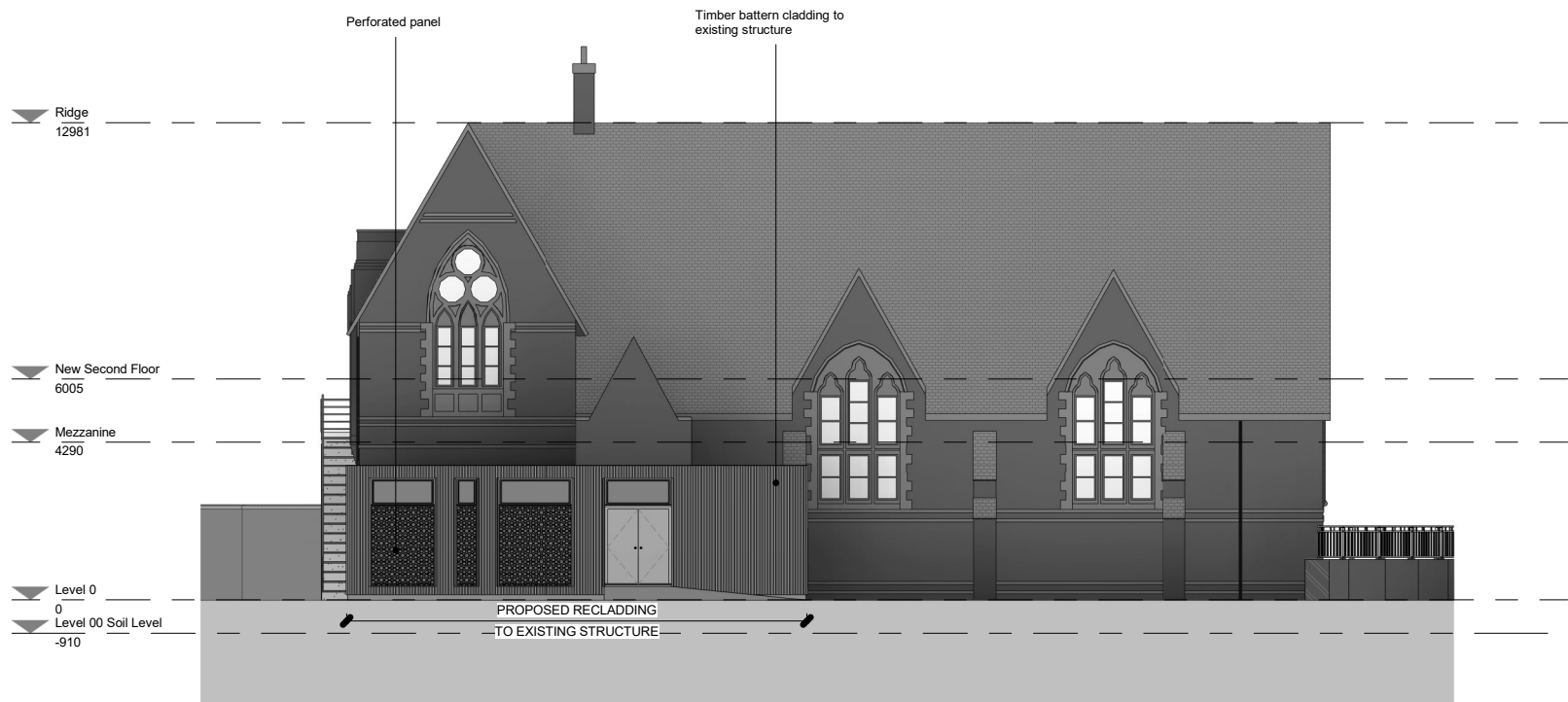
2 Proposed East Elevation 1 : 100
