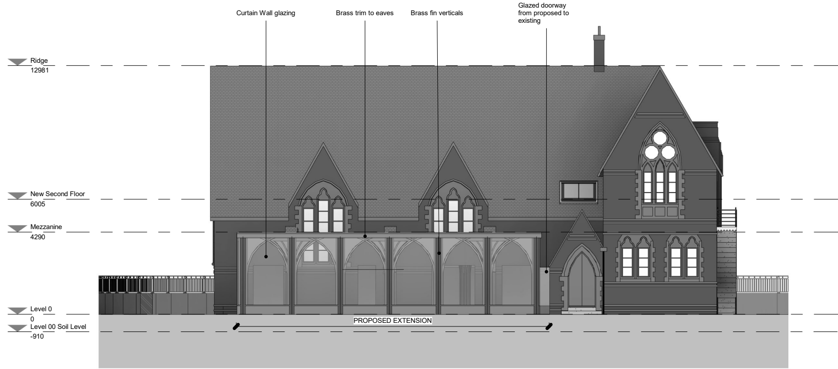
1 Proposed West elevation 1 : 100
