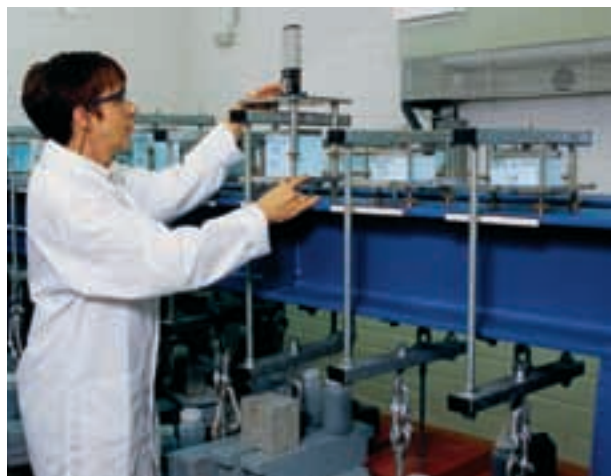
Fig. 10 » Creep testing STYROFOAM™ in the laboratory
