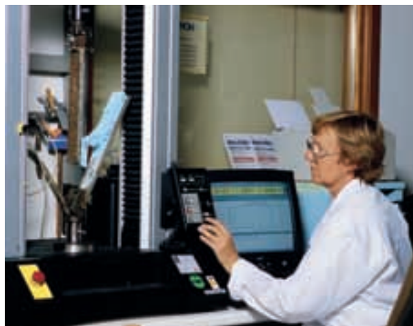
Fig. 11 » Shear test on STYROFOAM™
