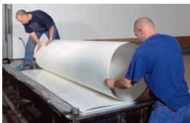
Fig. 09 >> Applying facing layer (GRP in this illustration)
