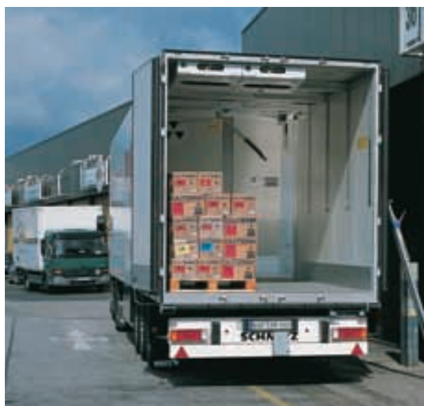
Fig. 14 » Well insulated and able to support loads: refrigerated truck bodies using STYROFOAM™ cored panels.
