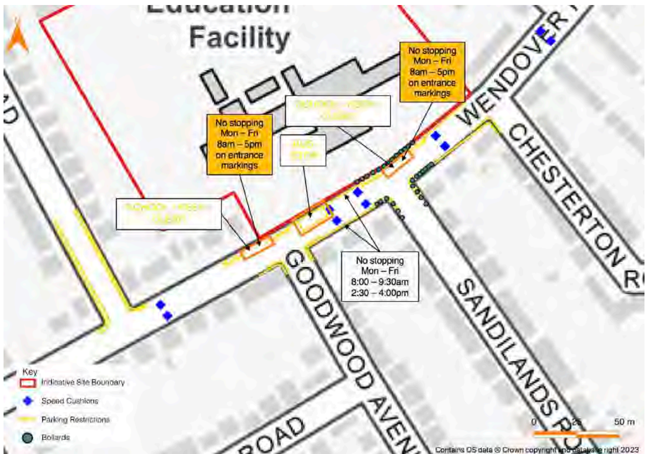
Figure 2.3 : Waiting Restrictions and Traffic Calming Measures on Wendover Road
