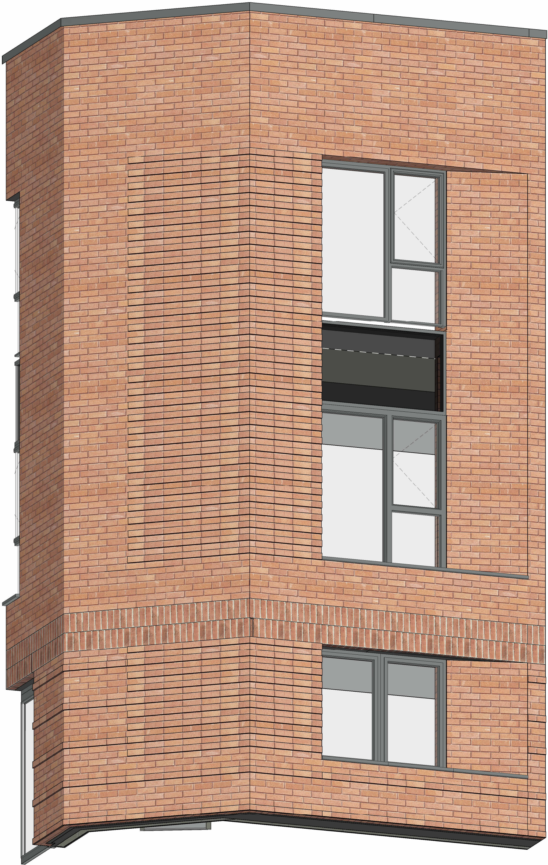
Indicative 3D - Corner Chamfered brickwork
