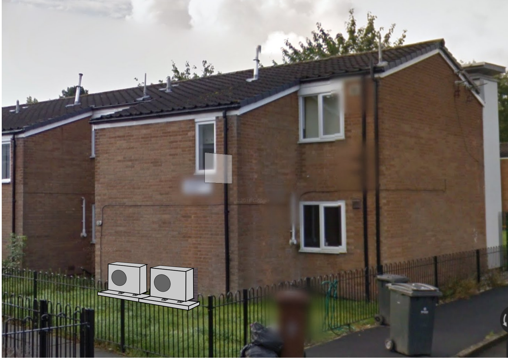
Proposed location of external heat pump serving heating and domestic hot water systems.
