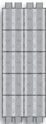
Typical Installation Channel Format 4 Clear Access Channels x 210mm
