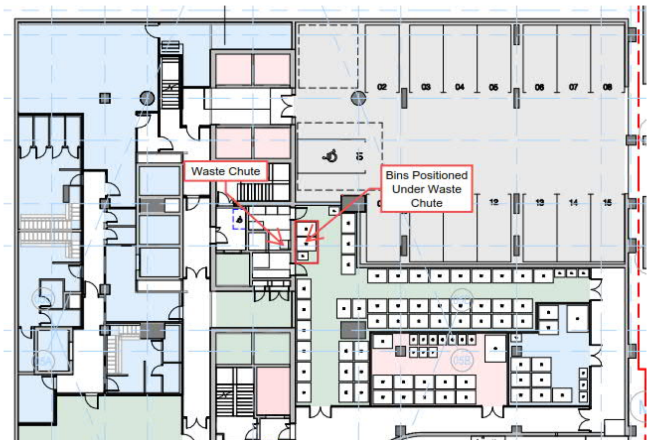
Figure 2-4 - Waste Chute Location (Basement Level)
