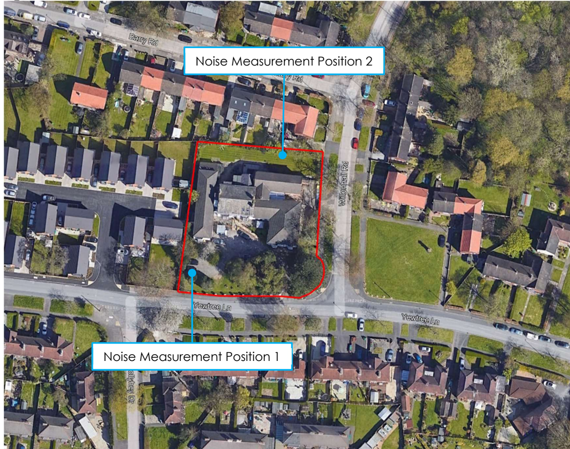
Figure 3.1: Baseline Noise Measurement Position
