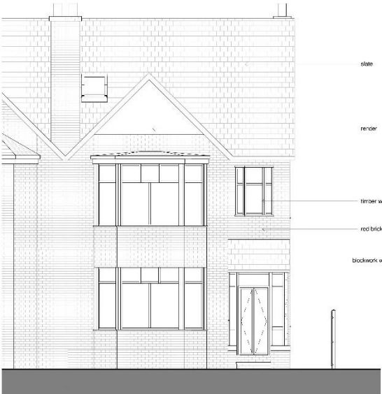
EXISTING ELEVATIONS - SOUTH 1 : 50
