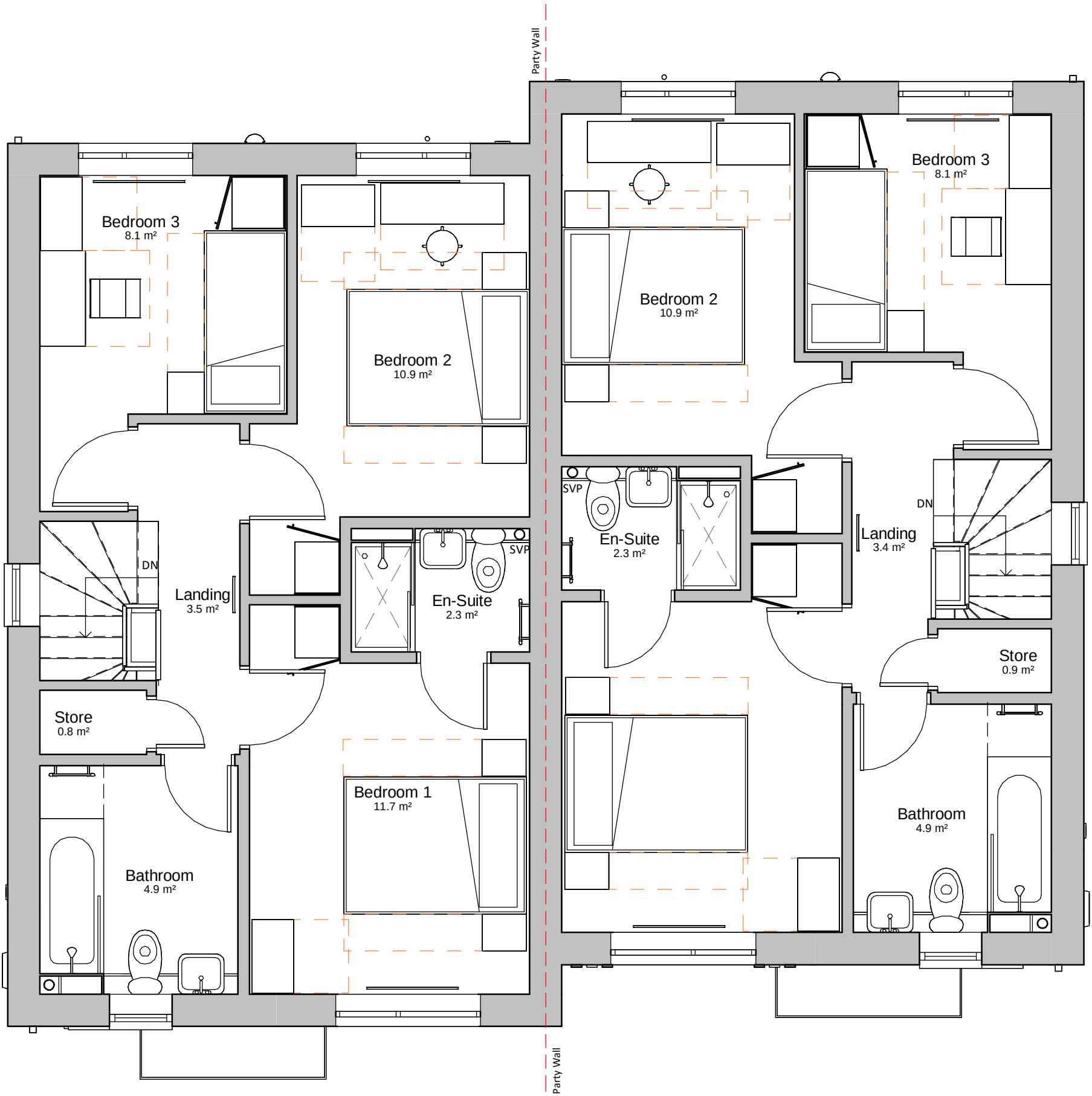
01 First Floor Plan (45m²) 1 : 50
