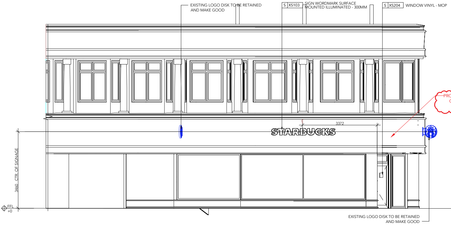
1 PROPOSED EXTERIOR ELEVATION - SHOPFRONT LHS. 1:100
