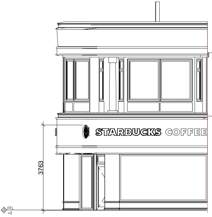
2 EXISTING EXTERIOR ELEVATION - SHOPFRONT RHS 1:100
