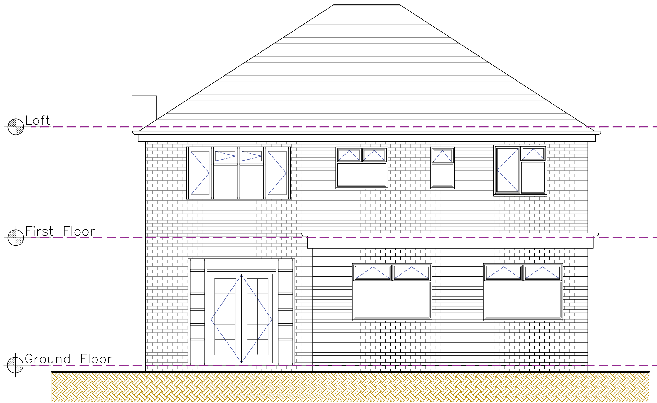
Existing Rear Elevation
