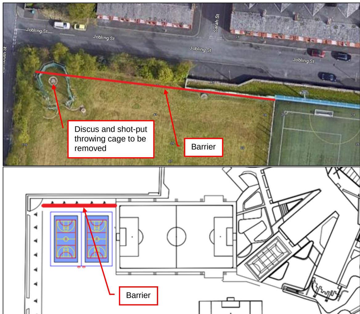
Figure 4.2 - Potential noise barrier location
