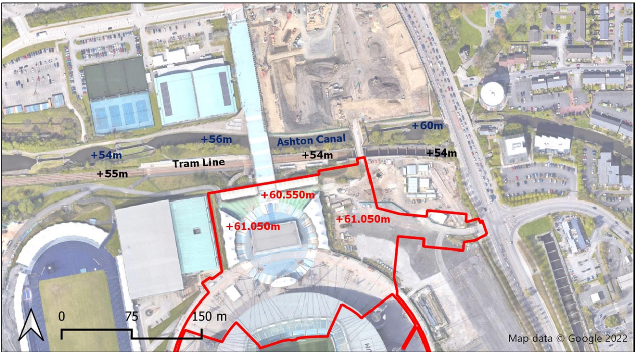
Figure 4—6 Levels between the Ashton Canal and the site.
