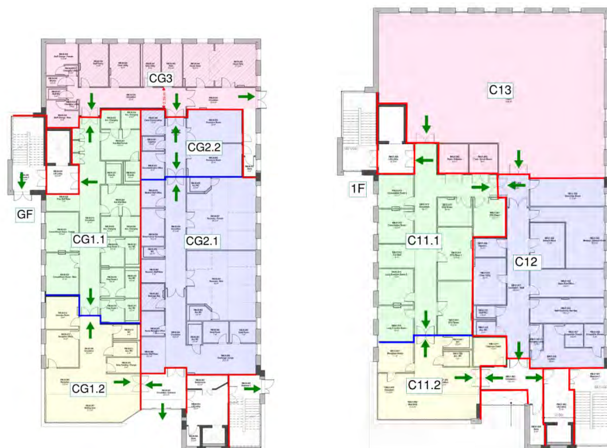
Figure 7: Compartment exits and compartment designs
