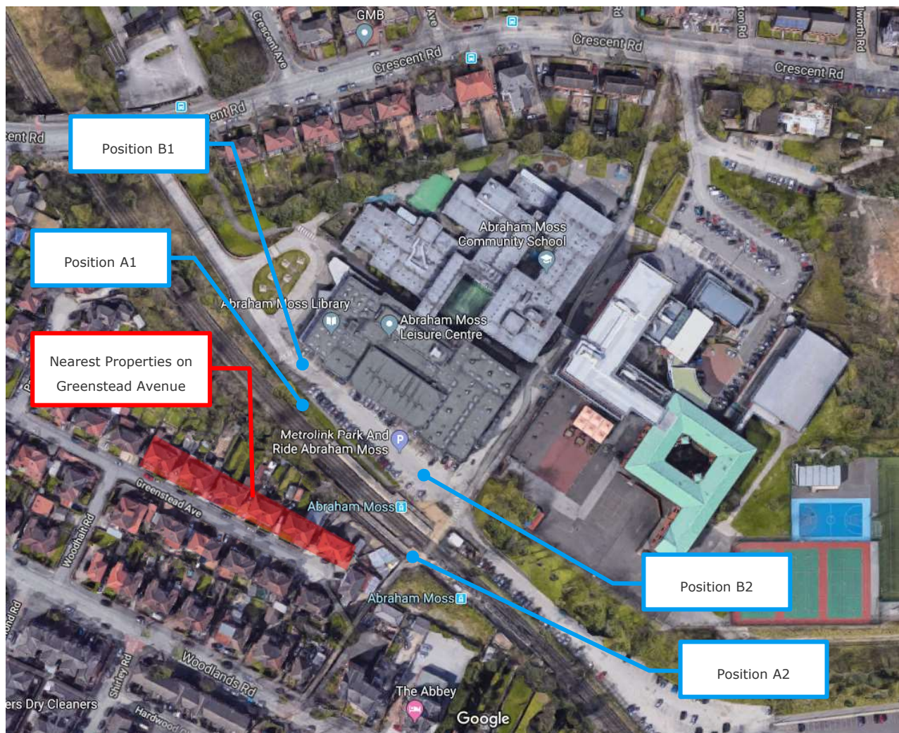
Figure 1 – Noise Measurement Positions and Results (old Leisure Centre shown but new centre is in a similar position)
