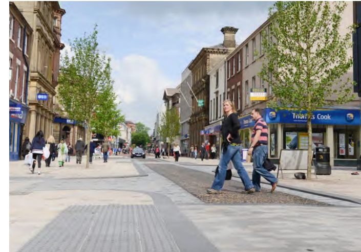
Low Kerbs, Street Trees, Quality paving materials & Crossing points
