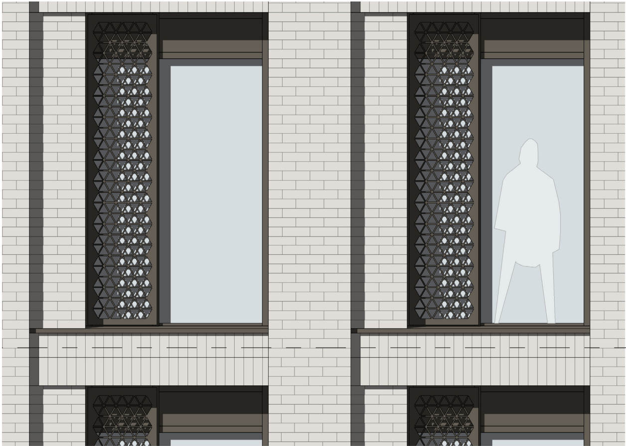
CARMOOR RD TYPICAL WINDOW ELEVATION
