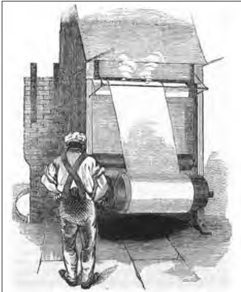
Plate 9: The singeing process, Penny Magazine 1843, 290
