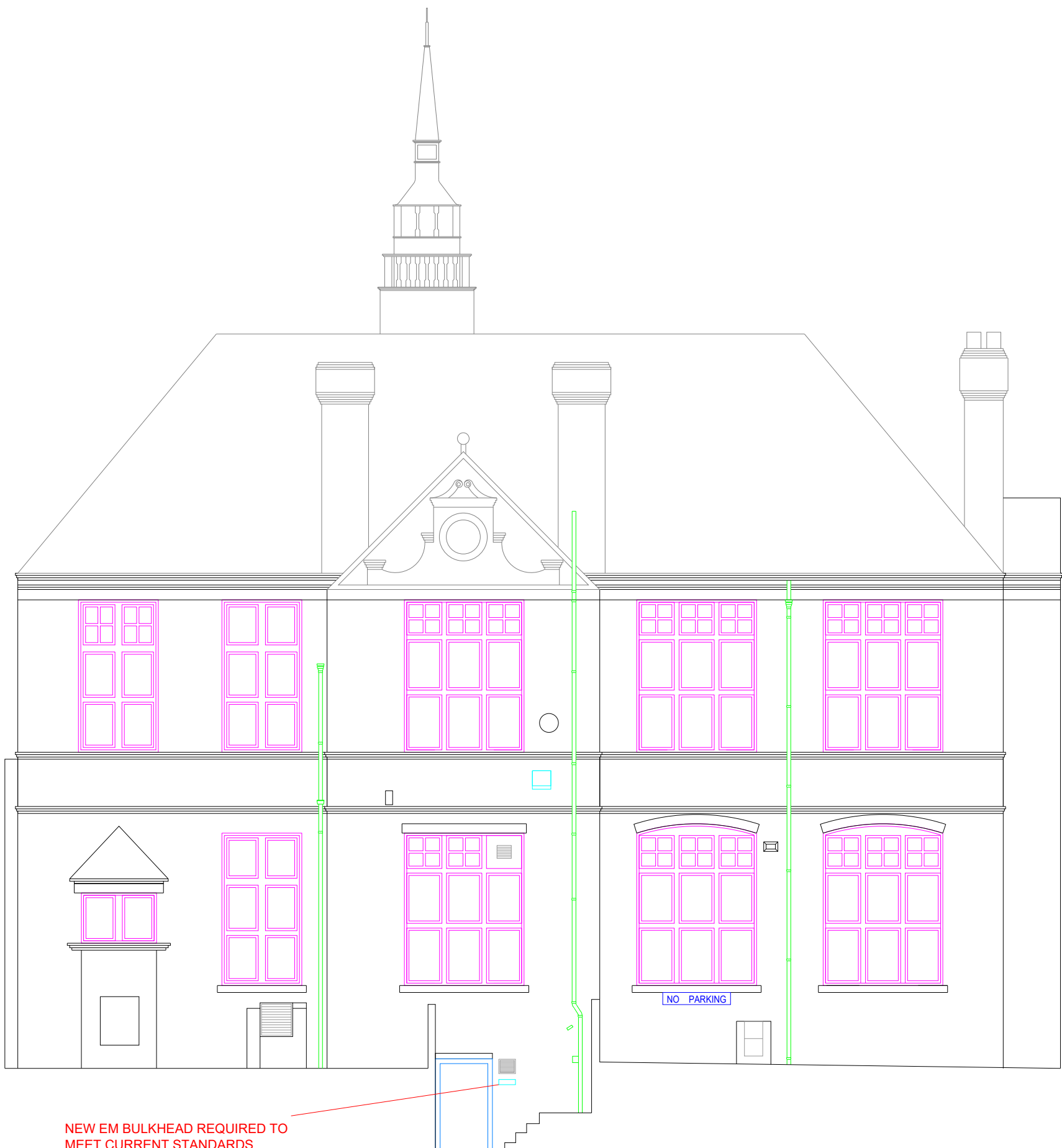
MAIN BUILDING - ELEVATION 2
