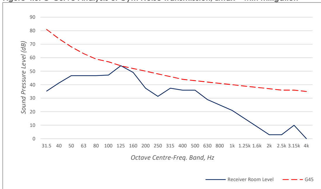
Figure 4.3: G-Curve Analysis of Gym Noise Transmission, Lmax – with mitigation
