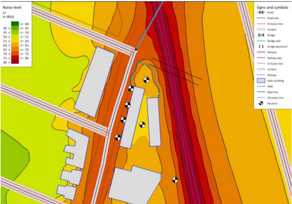
Site plan view of acoustic noise levels (taken from Acoustic Assessment)
