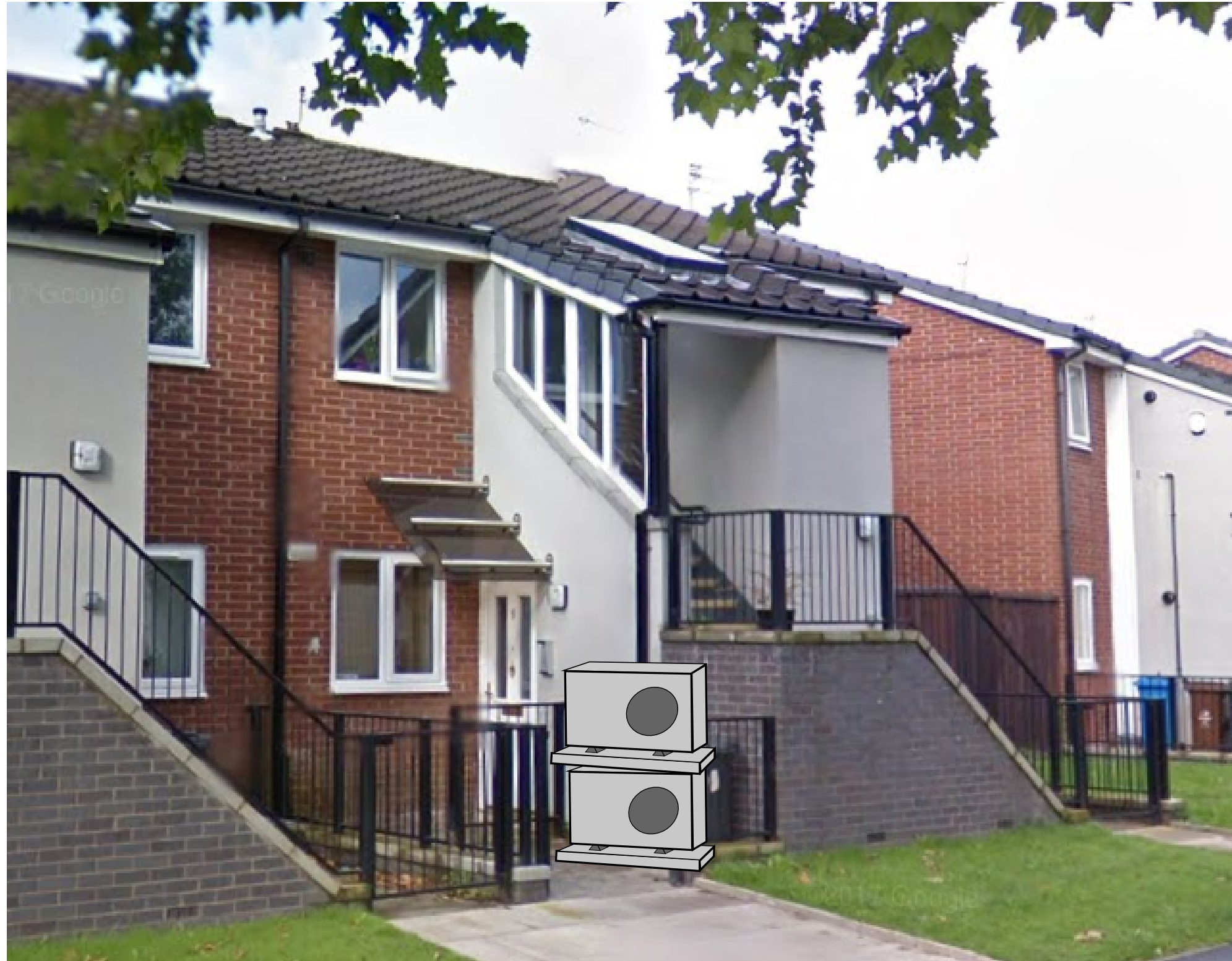
Proposed location of external heat pump serving heating and domestic hot water systems.
