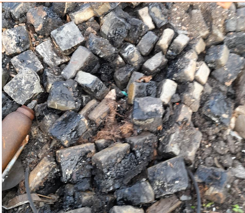
PLATE 4 COAL TAR SEALANT ON REMOVED COBBLES
