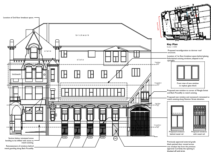
IMAGE 7: Proposed Back Piccadilly elevation showing the reinstated windows and escape door.
