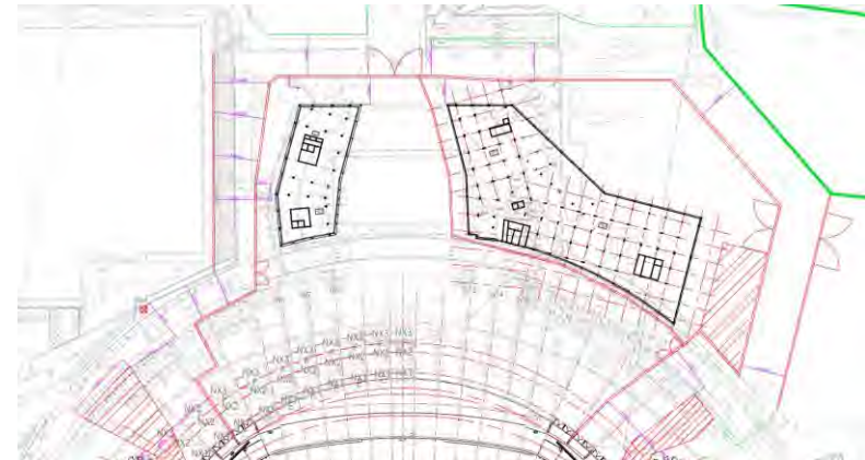
Figure 02: Proposed North Stand construction hoarding (Source: LOR)
