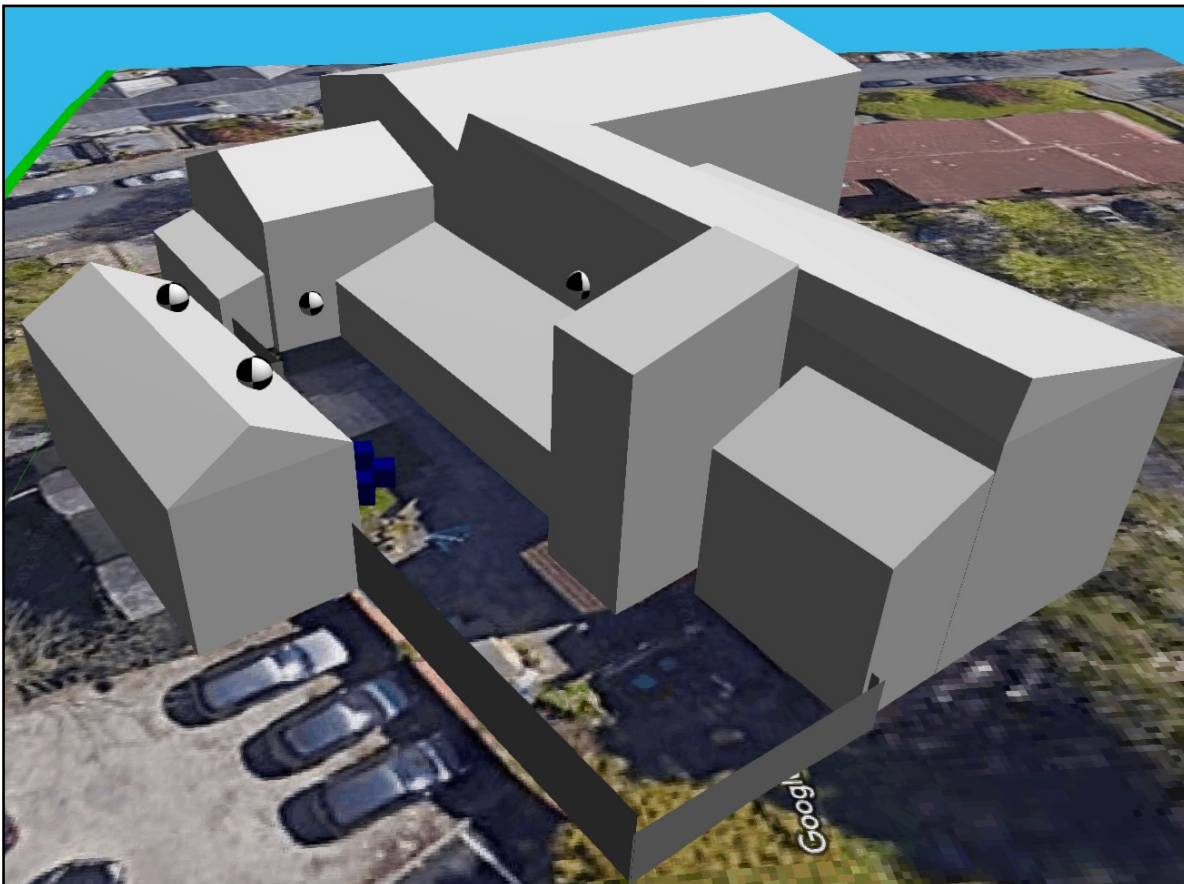
Figure 5.1: CadnaA Noise Propagation Model 3D View
