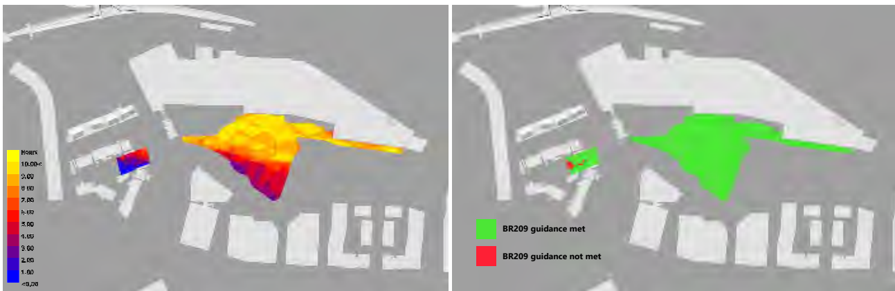
Figure 8 Sunlight distribution and BRE pass/fail on March equinox – amended Phase 1 and Mayfield masterplan buildings
