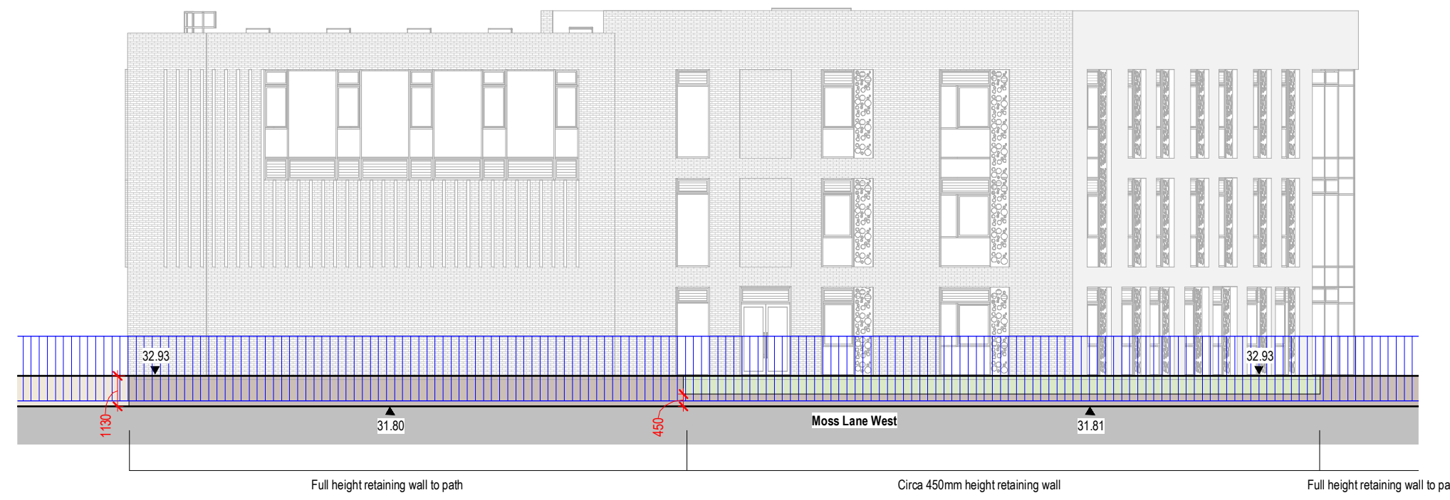
1 Retaining Wall Elevation 1 : 200 Ref Sheet: 9007
