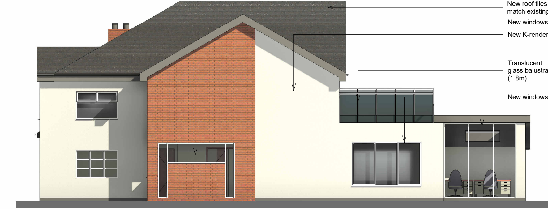
PROPOSED EAST ELEVATION 1:100
