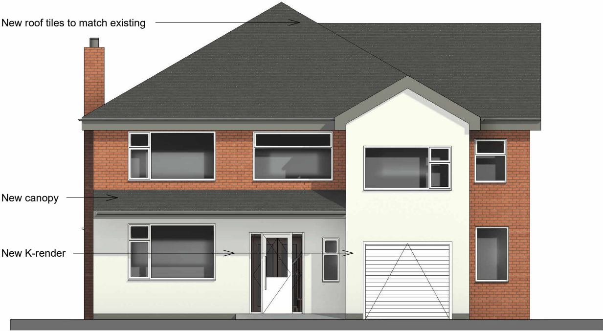
PROPOSED SOUTH ELEVATION 1:100
